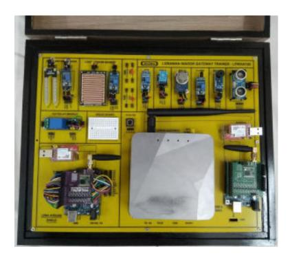
This trainer has been designed with a view to provide practical and experimental knowledge of Internet of Things (IOT) with LoRaWAN Outdoor Gateway Communication Sensors programing with Arduino IOT Boards with LoRaWAN Gateways.
