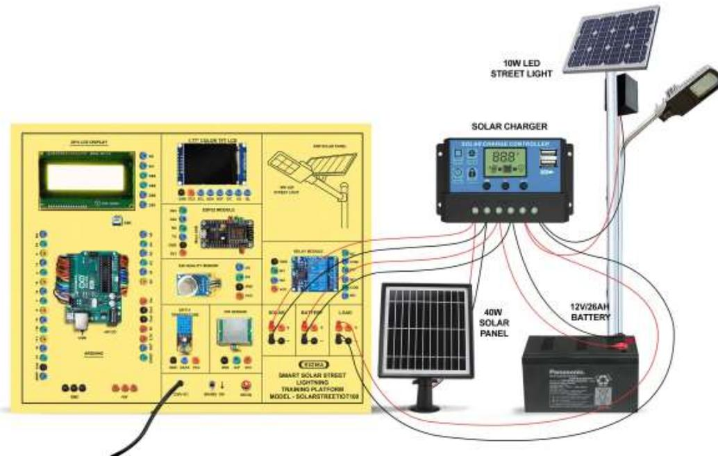
This trainer has been designed with a view to provide practical and experimental knowledge Sensors programming for IoT based Smart Solar Street Light system with Arduino IOT Board.
